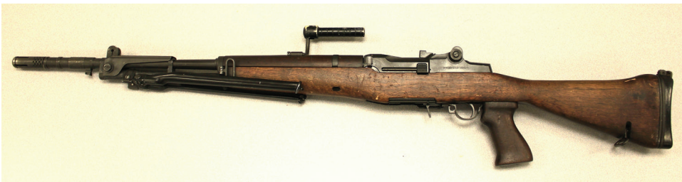
Figure 4.57 The M14-pattern rifle manufactured by Beretta as the BM59. There are definite similarities, but note the distinct differences between the M14 and the BM59. This example has a bipod, a grenade-launcher spigot on the muzzle, a grenade-launching ladder-type sight, and a pistol grip instead of a standard rifle stock. (Image from author's collection.)
